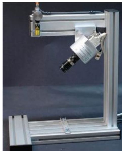
A ZPS-1000 laser scanning 3D measurement system from Z-Laser. The specialised camera and scanning lasers are held at a fixed angle, and objects to be imaged are moved beneath the system (typically by a conveyor). Image courtesy of Alrad Instruments.
